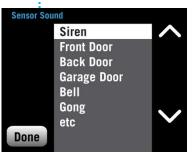
**Sensor Sound:** A custom sound can be added to each sensor. If this sensor is in alarm the selected sound will repeat three times before system siren begins. This provides audible recognition of which sensor has been tripped. When highlighted a sample of the sound is emitted. Siren is the main system siren sound. Push Done.
